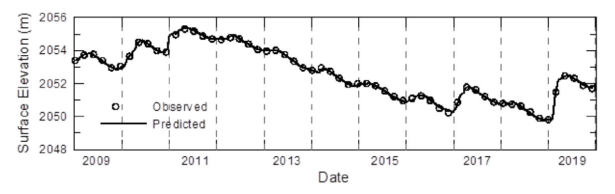
• With fitting of inflows, water levels were very accurately reproduced by model (MAE= 3.6 cm)
